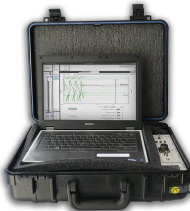
This portable system is based on a precision analog to digital converter controlled by a notebook computer with Windows-based application.
