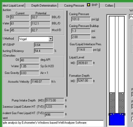
The Echometer Well Analyzer is used in conjunction with a gas gun/microphone assembly to determine the liquid level depth in a well. Normally, the liquid level depth is determined in the casing annulus, but also, the liquid level depth can be measured inside tubing in gas wells.
